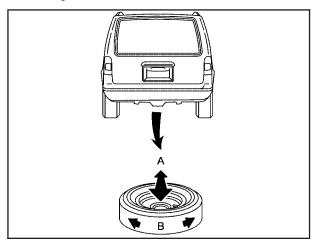
6. Make sure the tire is stored securely. Push, pull (A), and then try to turn (B) the tire. If the tire moves, use the wheel wrench and socket end of the extension to tighten the cable. 7. Return the equipment to the proper location in the vehicle as shown next.
