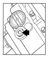
To get an accurate reading, the vehicle should be on a level surface. If the level is below the bottom of the filler plug hole, located on the transfer case, you'll need to add some lubricant. Add enough lubricant to raise the level to the bottom of the filler plug hole. Use care not to overtighten the plug.
