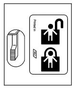
Move the lever down to engage the security lock. Move the lever up to disengage the security lock.
