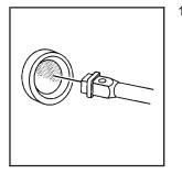
11. If the spare tire is hanging from the cable, insert the socket end of the extension connected to the wheel wrench into the hoist shaft hole just above the rear bumper on a 45 degree angle downward.
