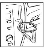
Your vehicle is equipped with a cupholder on the instrument panel next to the radio. To open the cupholder, push once on the arm and the cupholder will move into position for use. To close the cupholder, lift the arm up towards the instrument panel.
