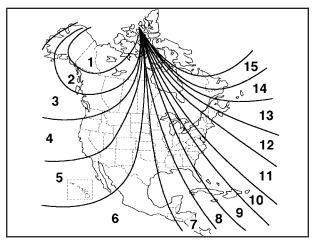
2. Press and hold the on/off button for six seconds. Release the button when ZONE is displayed. The number shown is the current zone number. 3. Scroll through the zone numbers that appear in the compass/temperature window on the mirror by pressing the on/off button. Once you find your zone number, release the button. After about four seconds, the mirror will return to the compass display, and the new zone number will be set.
