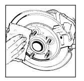
7. Remove any rust or dirt from the wheel bolts, mounting surfaces and spare wheel. 8. Place the spare tire on the wheel-mounting surface.
