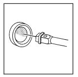
Insert the socket end of the extension (C) on a 45 degree angle downward into the hoist drive shaft hole. It is exposed when the rear gate is open and is just above the rear bumper.
