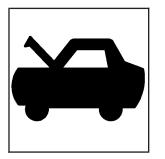
To open the hood, first pull the handle with this symbol on it. It is located inside the vehicle under the instrument panel on the driver's side.
