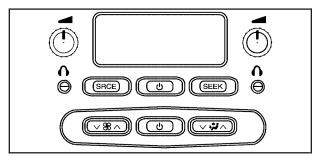
(**Power**): Press this button to turn the RSA on or off. The rear speakers are muted when the power is turned on.
