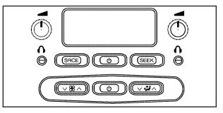
$\vee \, \Re \, \wedge \,$  (Fan) Press this button to adjust the fan speed.
