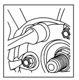
Using the wheel wrench, loosen all the wheel nuts. Do not remove them yet.
