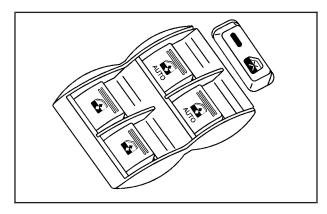
The controls for the power windows are located on the armrest on each of the side doors. With power windows, the switches operate the windows when the ignition is in RUN, ACCESSORY or when Retained Accessory Power (RAP) is active. See *Retained Accessory Power (RAP)* on page 2-21. The driver's door also has a switch for each of the passenger's windows.
