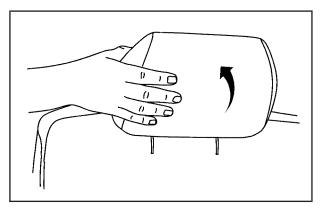
To return the head restraint to the upright position, reach behind the seat and pull the restraint up until it locks into place. Push and pull on the head restraint to make sure that it is latched securely.
