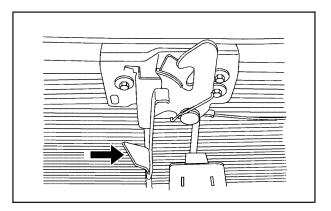
2. Then go to the front of the vehicle and push the secondary hood latch up and to the right to release it, then lift the hood.
