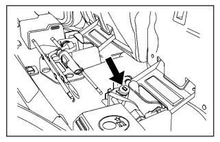
To release the jack from its holder, turn the knob on the jack counterclockwise to lower the jack head.
