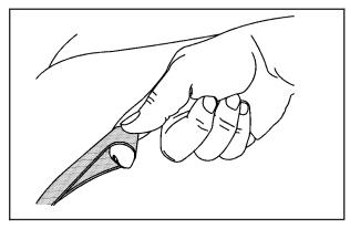
Pull up on the loop located where the seat cushion meets the seatback to fold the seat cushion up and out of the way. This will allow the seatbacks to fold flat and increase the cargo area.
