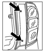
2. Remove the screws from the taillamp assembly.
