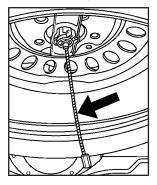
Check under the vehicle to see if the cable is visible. If it is not visible, proceed to Step 6.
