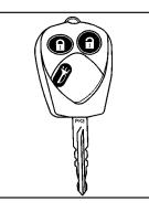
Your vehicle is equipped with the PASS-Key<sup>®</sup> III (Personalized Automotive Security System) theft-deterrent system. PASS-Key<sup>®</sup> III is a passive theft-deterrent system.
