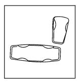
The power seat controls are located on the outboard side of the front seat cushions. The horizontal control adjusts the seat cushion and the vertical control adjusts the seatback. **Power Lumbar**
