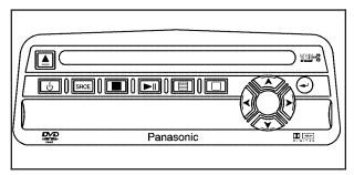
(**Power**): Press this button to turn the RSE system on and off. The power indicator light will illuminate when the power is on.
