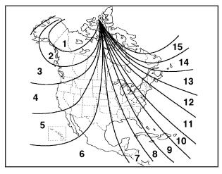
2. Press and hold the on/off button for six seconds. Release the button when ZONE is displayed. The number shown is the current zone number.  Scroll through the zone numbers that appear in the compass/temperature window on the mirror by pressing the on/off button. Once you find your zone number, release the button. After about four seconds, the mirror will return to the compass display, and the new zone number will be set.
