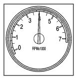
The tachometer displays the engine speed in revolutions per minute (rpm).
