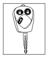
**d** (Unlock): Press the unlock button to automatically unlock the driver's door. The parking lamps may flash and the interior lights will go on. Press the unlock button again and all remaining doors will unlock.
