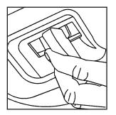
You should adjust the steering wheel before you drive. The tilt lever is located to the left of the steering column, under the turn signal lever.
