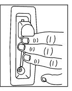
The rear seatback levers are located on the outboard side of each rear seatback.
