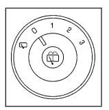
This control is located to the left of the steering wheel on the instrument panel. To turn the rear wiper on, turn the control to either 1, 2, or 3. For delayed wiping, turn the control to 1 or 2. For steady wiping, turn the control to 3. To turn the wiper off, turn the control to 0.
